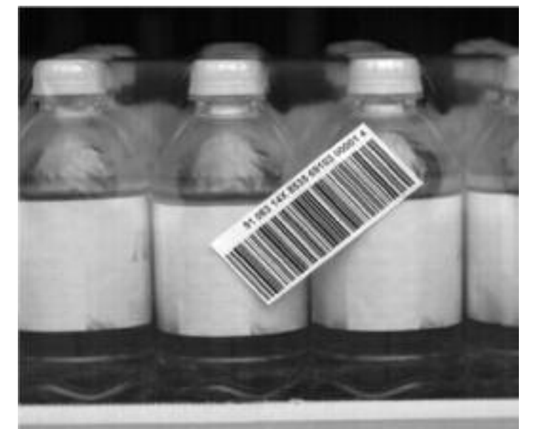
BP850 separates the outer shipping label from the product labels.
