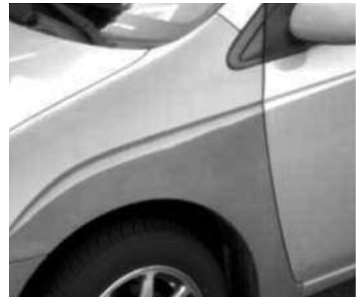
BP324 Machine Vision Filter shows a mismatch in the clear coat.
